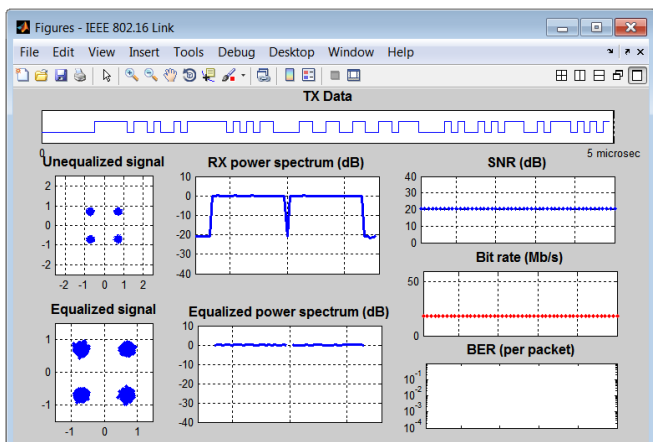
Fig.8 Effect on received and equalized signal when there is no fading.
