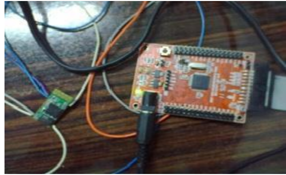
Fig. 9: Transmitter Module of Wireless Monitoring System Above Fig. 8 shows the real-time Model of portable Wireless transmitter Module.
