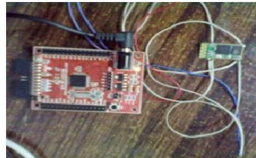
Fig. 10 Receiver Module of Wireless Monitoring System
