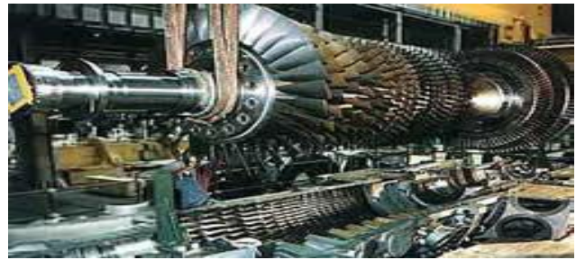
Fig.5. Large steam turbines require creep-resistant steels for safe, economical operation.
