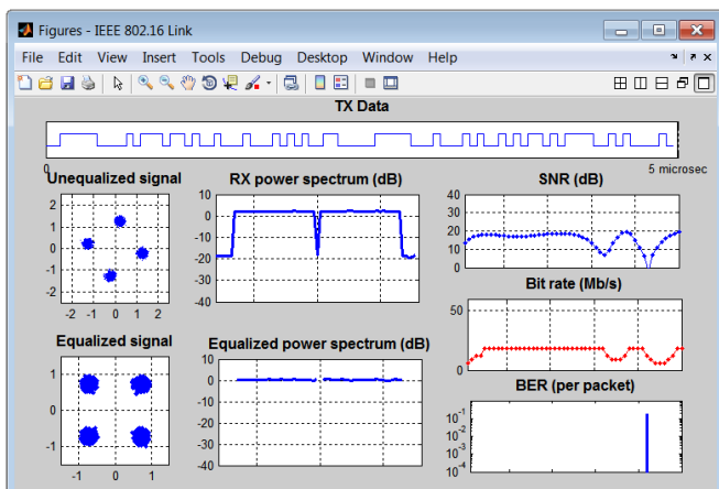
Fig.9 Effect of flat-fading channel on received and equalized signal
